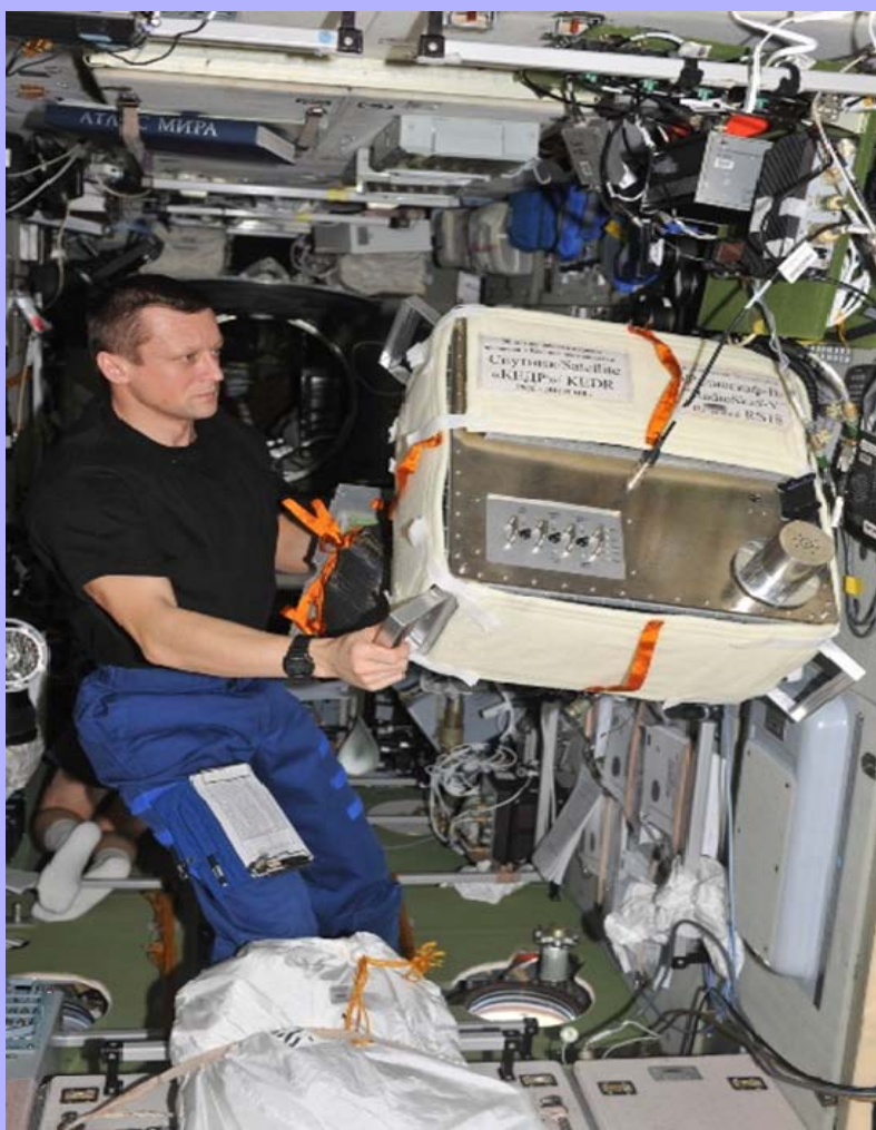
ARRISat-1 as seen inside the International Space Station on February 10th 2011 being moved around by Russian Cosmonaut Dmitry Kondratyev. The VHF port of ARRISat, which is normally connected to a Kapton protected 1/4 wave monopole was connected to one of the external antennas that exist on the Station. The grab handles provided by AMSAT-UK for this project can be clearly seen in this photograph!
