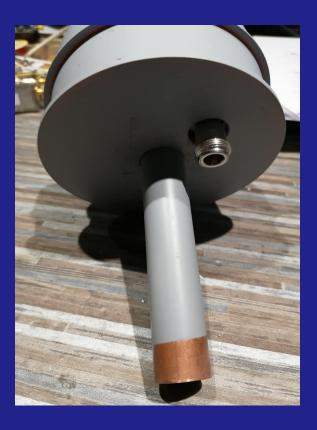
A feed for 2400 MHz LHCP (single or separate RX/TX antenna)
