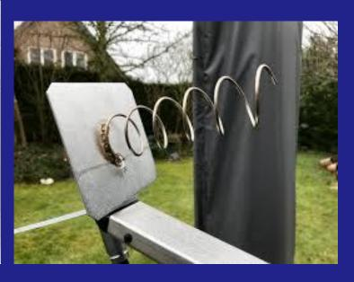
A feed for 2400 MHz LHCP (single or separate RX/TX antenna)
